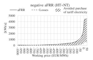
Fig. 11. Coincidence of aFRR purchase and resulting thermal losses (Brennenstuhl, Pietruschka, Yadack, & Eicker, 2017).
