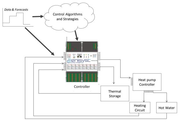
Fig. 1. Control scheme on building level
