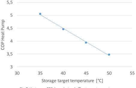
Fig. 7. Heat pump COP dependent on buffer storage temperature
