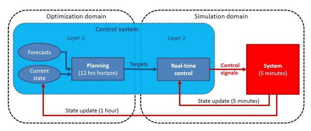
Fig. 15. Schematic overview of the advanced control logic. (Vivian, Jobard, Ben Hassine, Pietrushka, & Hurink, 2017)
