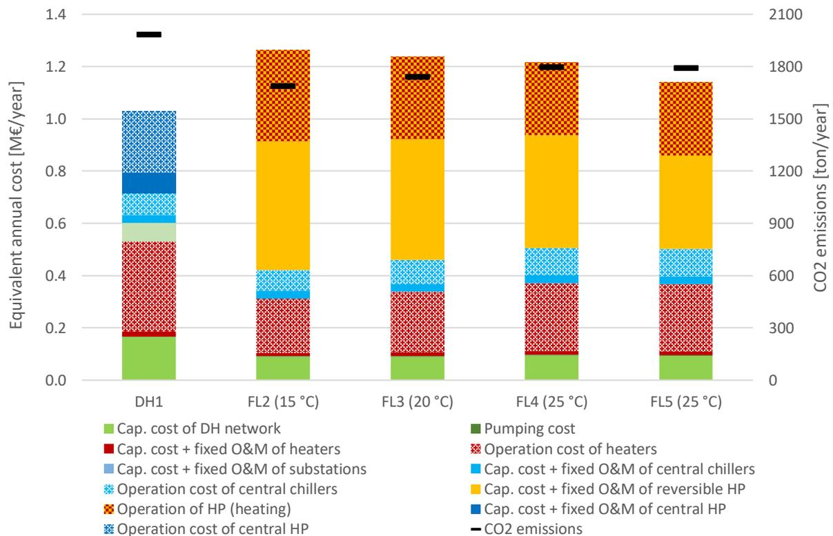
Figure 17: Composition of the equivalent annual cost and CO<sub>2</sub> emissions in the scenarios DH1, FL2, FL3, FL4 and FL5.
