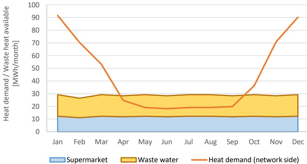
Figure 10: Yearly profile of the heat demand on the network side and of availability of waste heat from the supermarket and from the waste water pipe. The values are expressed in terms of amount of heat per month.
