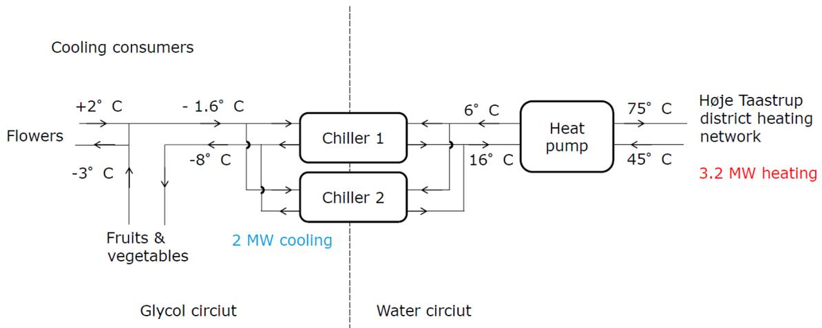
Figure 14: Principle scheme of the interface between the cooling consumers at the Copenhagen markets and the Høje Taastrup DH network: compression chillers and heat pump (Rambøll, 2017).
