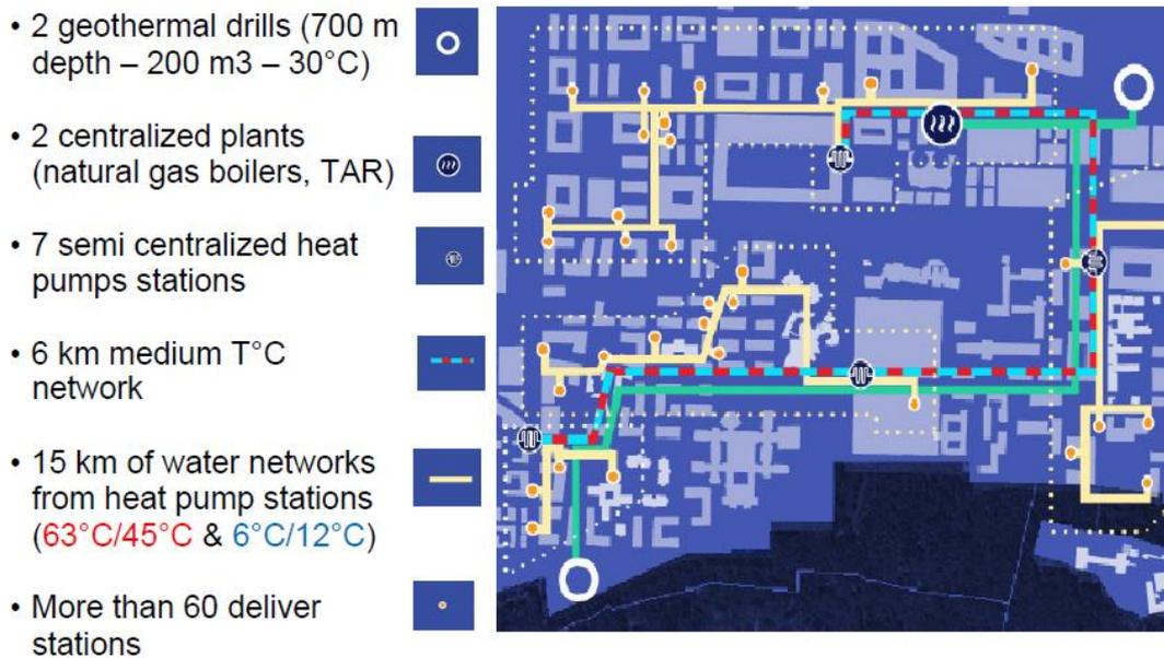
Figure 3 – Sub-systems of the Paris-Saclay DHC system <sup>(3)</sup>
