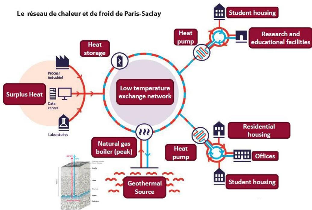
Figure 4 – General principle of the smart DHC network of Paris Saclay <sup>(4)</sup>
